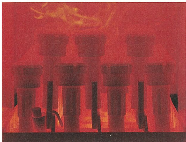
Heat-treatment furnace for drill bits. Extensive material and process know-how forms the basis of our high product quality.
