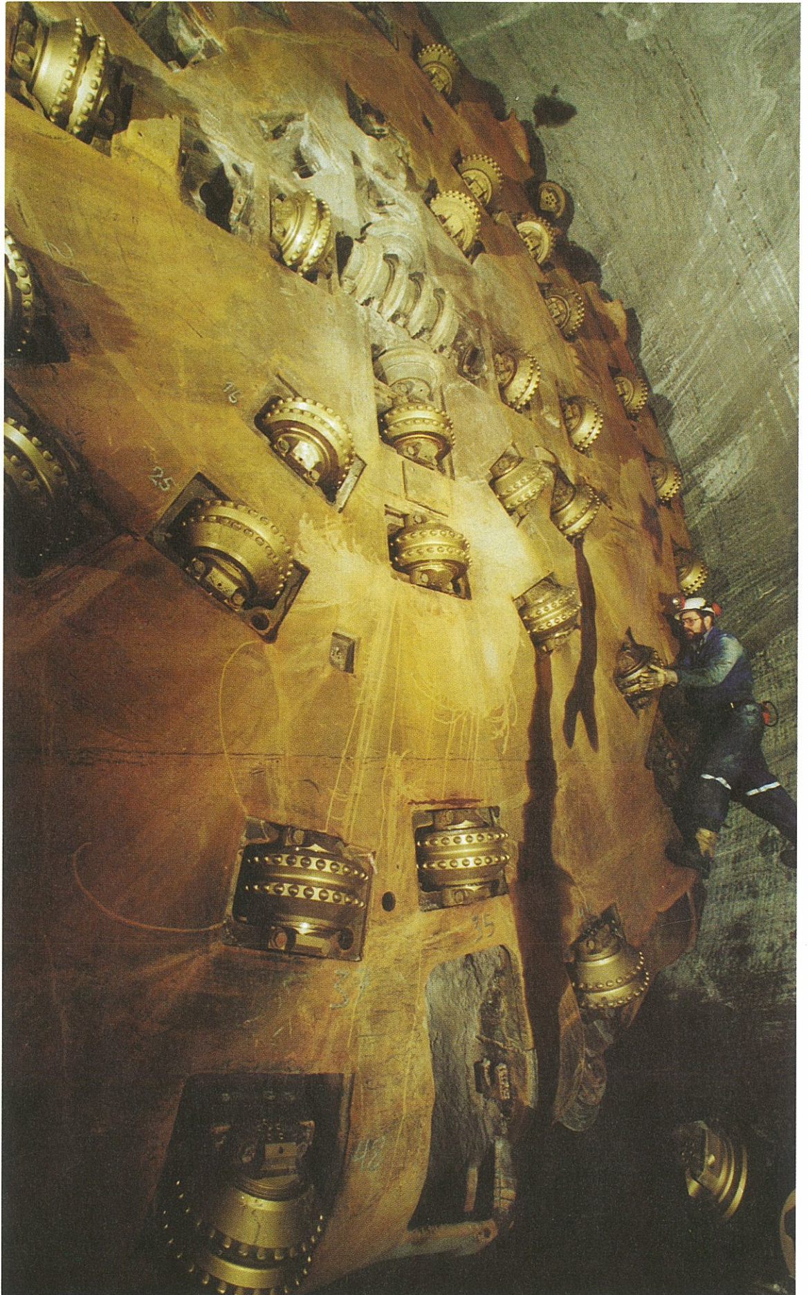
Sandvik's new carbide rollers on an 8.5-metre tunnel-driving machine being used on a power-station project under Svartisen in Norway.
