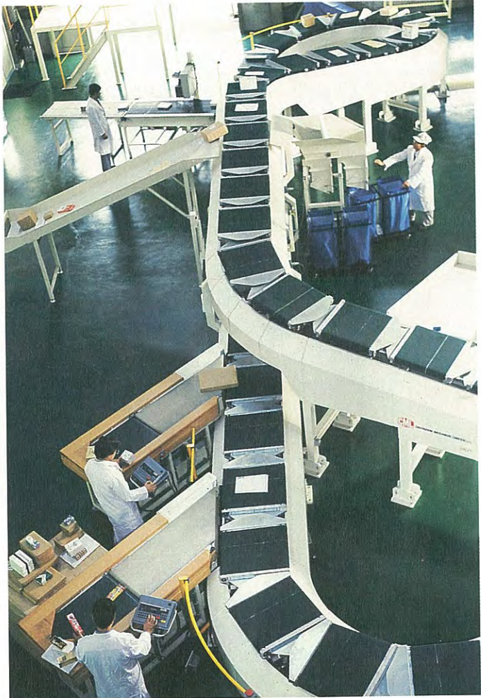
A DEMONSTRATION SET-UP FEATURING CML'S SYSTEM FOR SORTING SMALL PARCELS.
