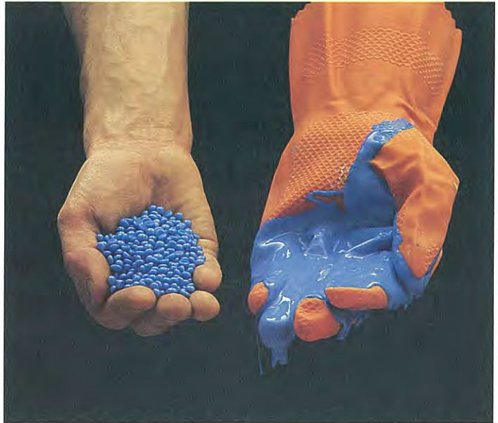
IN THE UNIQUE ROTOFORM PROCESS, MOLTEN MATERIAL RIDING A STEEL BAND IS TRANSFORMED INTO EASILY HANDLED PASTILLES.
