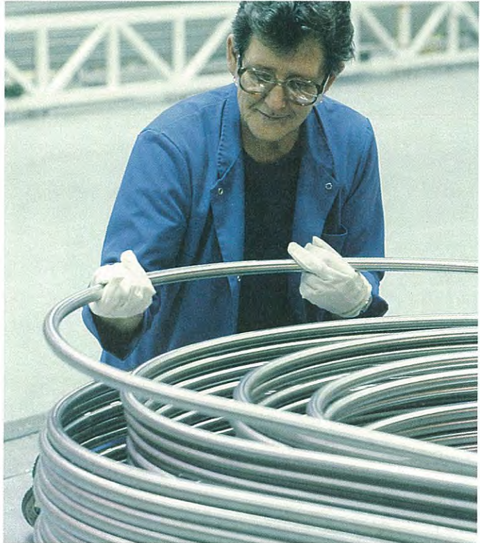
STEAM-GENERATOR TUBES FOR NUCLEAR POWER PLANTS MAKE HEAVY DEMANDS ON THE PROPERTIES OF THE STAINLESS STEEL.
