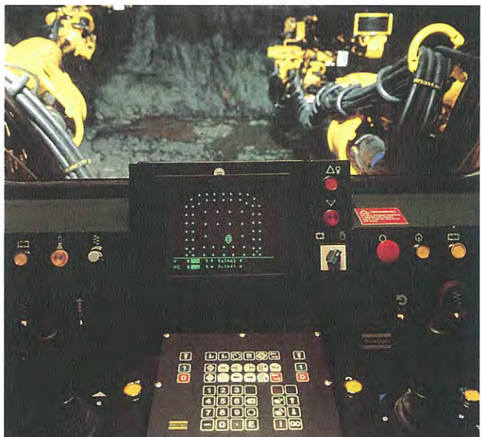
A COMPUTERIZED DRILLING RIG, THE ATLAS COPCO ROBOT BOOMER, FOR THE UNMANNED DRILLING OF BLAST-HOLES IN TUNNELLING.
